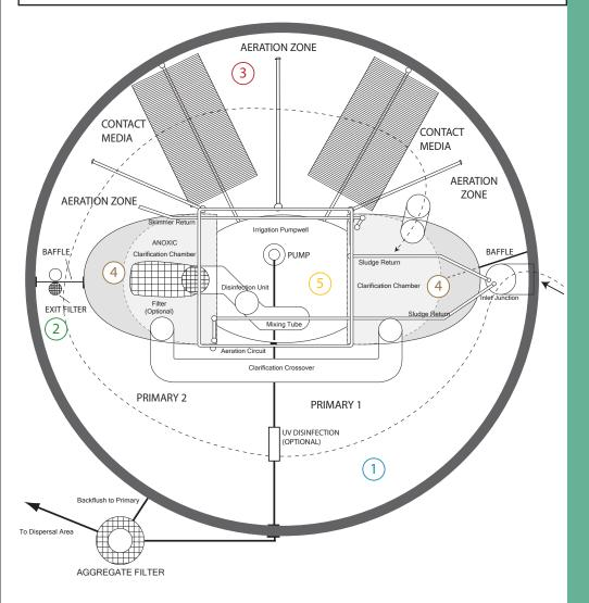
(At this stage an aggregate filtration unit can be fitted to upgrade discharge quality to 'advanced secondary' if required).
